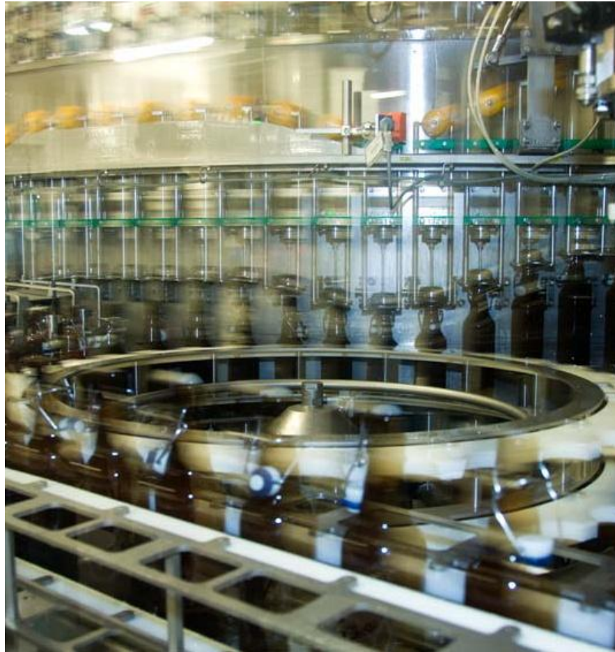
Container infeed on the KRONES Sensometric filler Output rate up to 72.000 container/h
